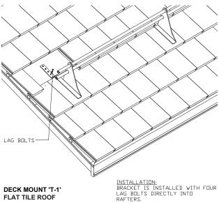
Fence bracket to be installed using (4) 3/8" x 4" (or longer) lag bolts fastened into roof truss, rafter, purlin or other structural roof member. Fasteners embed into structure with a 3" minimum. All roof penetrations that go through the underlayment are required to be flashed or sealed.
