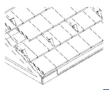
Bracket hooks to upper end of roof tile and counter batten. Bracket is installed with triangular end of bracket at butt end of roof tile and upper end under the course above.
