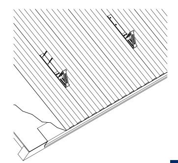
Bracket installed using (2) #14 screws fastened through roof material and sheathing below. Bracket installed with triangular portion of bracket towards roof eave.
