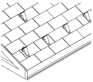
INSTALLATION: BRACKET IS INSTALLED WITH TWO 2-1/2" SCREWS WITH TRIANGULAR END OF BRACKET AT EAVE END OF ASPHALT SHINGLE.
