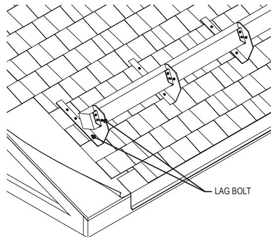
Fence bracket to be installed using (4) 3/8" x 4" (or longer) lag bolts fastened into roof truss, rafter, purlin or other structural roof member. Fasteners embed into structure with a 3" minimum. (2) Lag bolts are also required to secure timber to fence bracket through tab provided.
