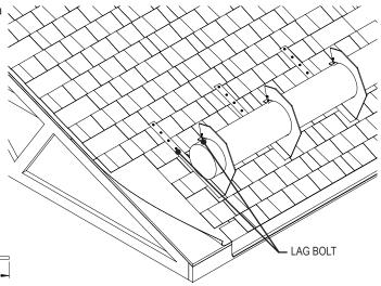
Fence bracket to be installed using (4) 3/8" x 4" (or longer) lag bolts fastened into roof truss, rafter, purlin or other structural roof member. Fasteners embed into structure with a 3" minimum. Lag bolt is also required to secure log to fence bracket through tab provided.
