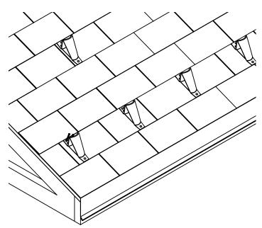
INSTALLATION: BRACKET IS INSTALLED WITH TWO 2-1/2" SCREWS WITH TRIANGULAR END OF BRACKET AT EAVE END OF ASPHALT SHINGLE.
