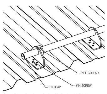
Snow Fence Bracket to be installed using (4) #14 fasteners secured to the purlins or roof sheathing. Space Snow Fence Brackets horizontally according to TRA Snow and Sun recommendations. Collars should be installed inside the last bracket and End Caps should be placed at pipe terminations.
