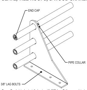
Snow Fence Bracket to be installed using (4) 3/8" Lag Bolts secured to truss, rafter, beam, or other structural member. Space Snow Fence Brackets horizontally according to TRA Snow and Sun recommendations. Collars should be installed inside the last bracket and End Caps should be placed at pipe terminations.
