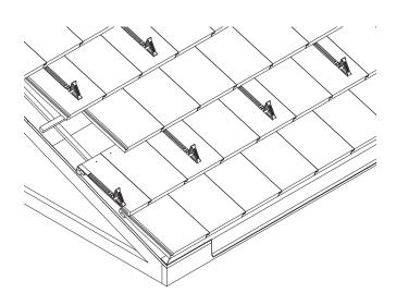
Bracket hooks to upper end of roof tile and counter batten. Bracket is installed with triangular end of bracket at butt end of roof tile and upper end under the course above.
