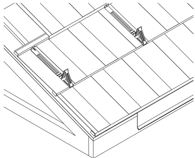
After metal tile has been installed on deck with 2"x2" batten, install the J bracket with the triangular end towards the down hill slope. Install a high quality construction adhesive below the triangular end of the bracket. Then install 3/16" screw into through hole in the snow bracket through hole in metal/granule tile into 2"x2" batten a minimum of 1 1/4".
