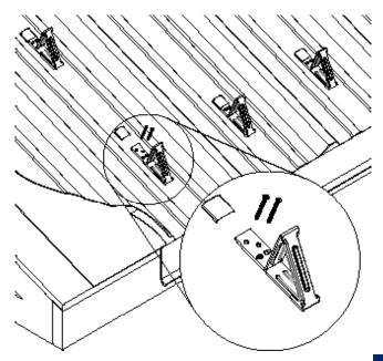
Bracket installed without clip use (2) #14 screws. Bracket installed with clip use (2) #8 screws. Screws must fasten through roofing material and sheathing below. Bracket installed with triangle portion of bracket downslope of roofing material.
