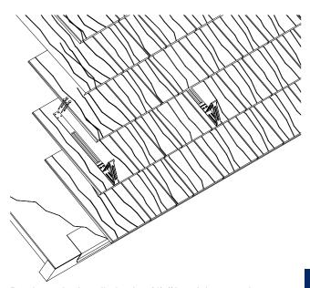
Bracket to be installed using (4) #8 stainless steel screws or roofing nails fastened through roofing material and sheathing below.
