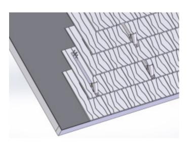
Bracket to be installed using (4) #8 stainless steel screws or roofing nails fastened through roofing material and sheathing below.
