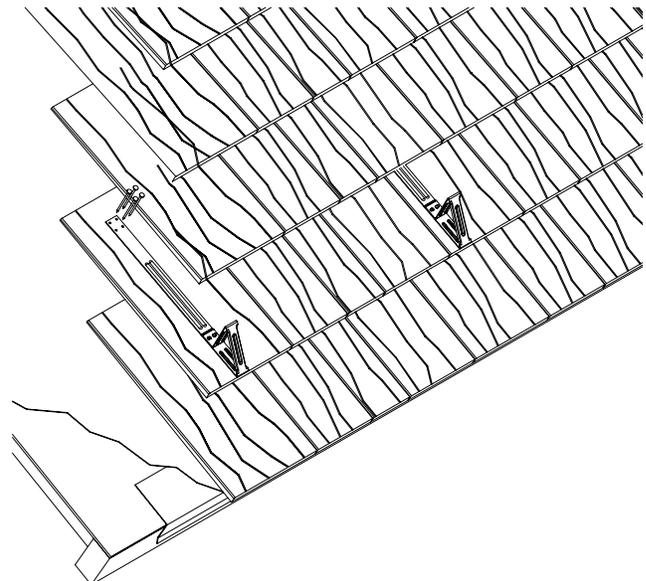
Bracket to be installed using (4) #8 stainless steel screws or roofing nails fastened through roofing material and sheathing below.
