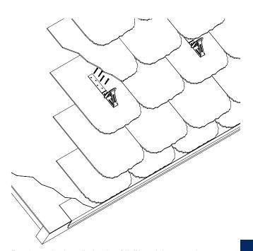
Bracket to be installed using (4) #8 stainless steel screws or roofing nails fastened through roofing material and sheathing below.
