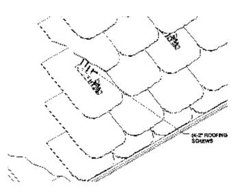
Bracket to be installed using (4) #8 stainless steel screws or roofing nails fastened through roofing material and sheathing below.
