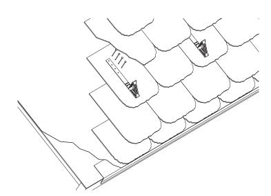
Bracket to be installed using (4) #8 Stainless Steel screws or roofing nails fastened through roofing material and sheathing below.
