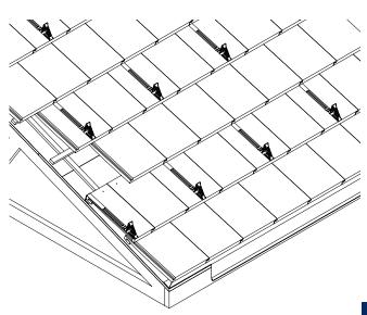
Snow Bracket hooks to upper end of roof tile and counter batten. Bracket is installed with triangular end of bracket at butt end of roof tile and upper end under the course above.
