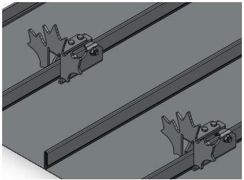
INSTALLATION: CLAMP THE SNOW FENCE TO THE RIB BY USING A TORQUE WRENCH WITH 30 FT - LBS. OF PRESSURE APPLIED TO EACH BOLT. FOR SPECIFIC ENGINEER-ING & PLACEMENT CALL TRA SNOW & SUN AT 801-756-8666.
