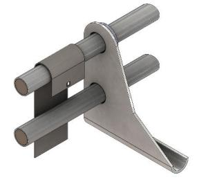
Snow Fence is installed with (4) 3/8"x 4"Lag bolts screwed into rafters/trusses, blocking or other structural framing. Locate trusses, position snow fence holes directly over center of truss, pre-drill holes to a depth of 4"using a 1/4"drill bit. We advise placing some type of caulking or sealant in the location of the holes before installing lags. Flashings can then be fabricated and placed at the installers discretion.
