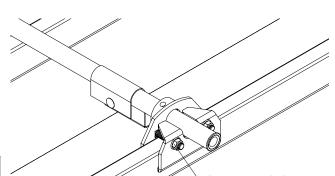
TIGHTEN WITH TORQUE WRENCH TO 30 FT LBS.
